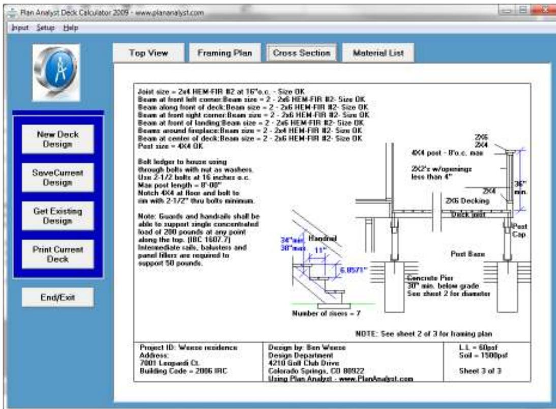
TO VIEW THE DRAWINGS, CLICK THE **TOP VIEW**, **FRAMING PLAN** OR **CROSS SECTION** TABS ABOVE THE DRAWINGS.
